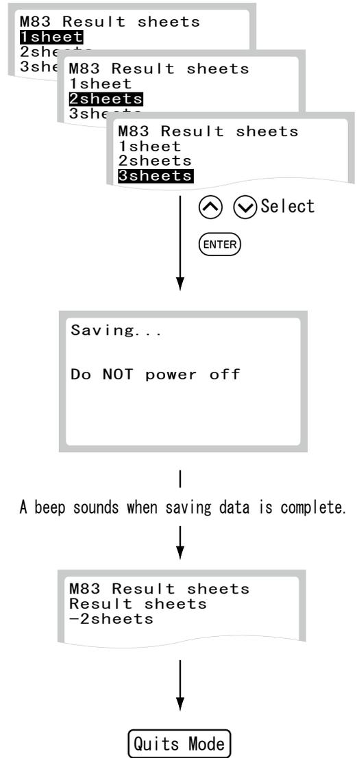
After the new setting for the print sheets is displayed, the analyzer quits the mode operation.
