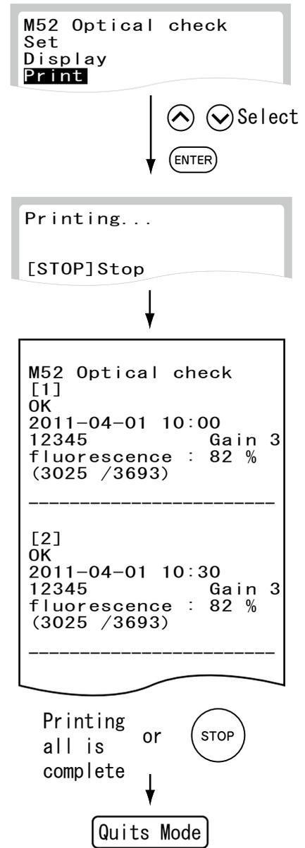
After printing the optical check result, the analyzer quits the mode operation.
