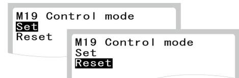
Select a menu using ▲ or ▼ whether to set or reset the control mode and press ENTER.
