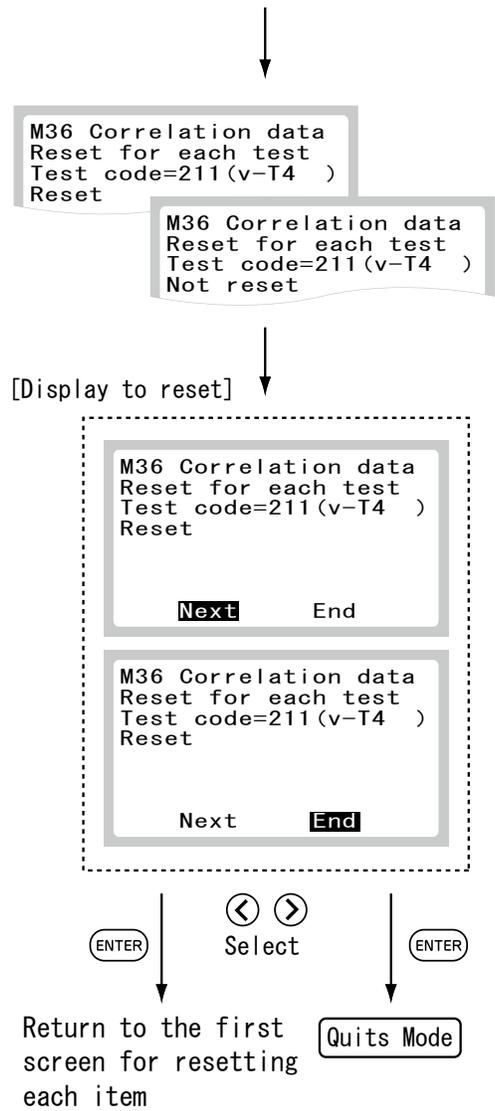
5. To reset coefficients for all tests:
