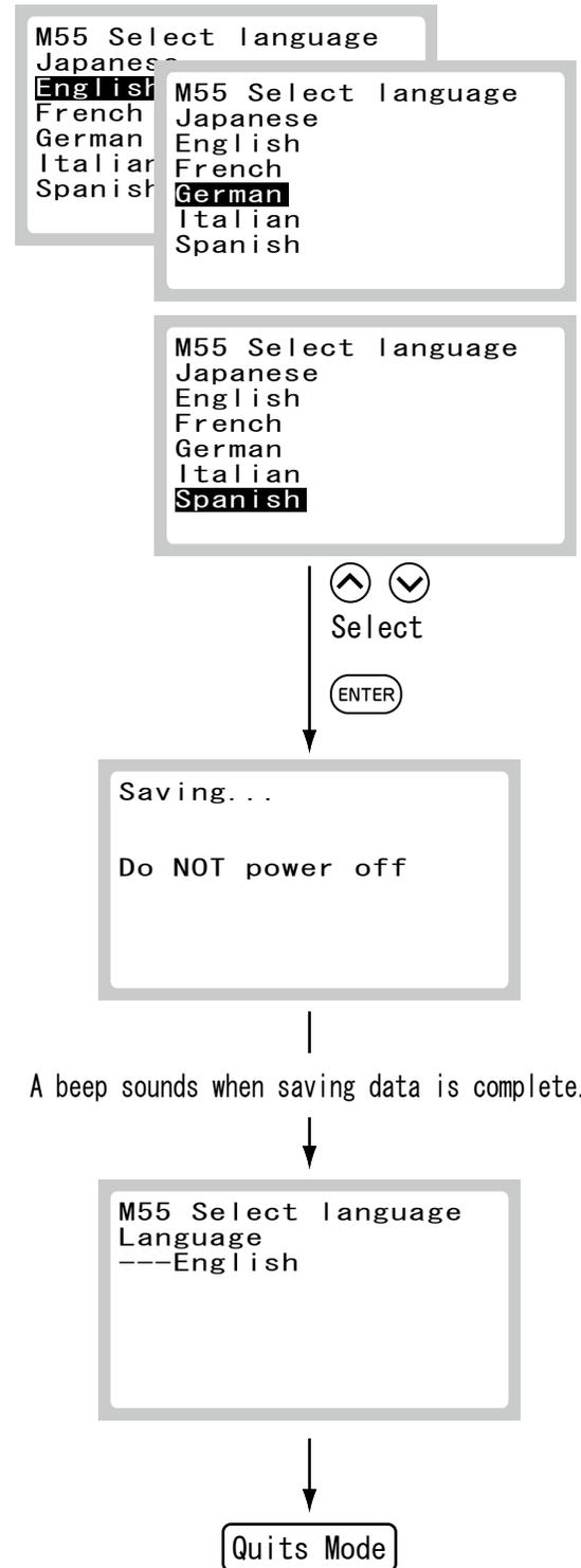
After the new selection is displayed, the analyzer quits the mode operation.
