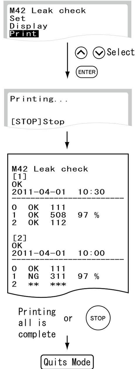
After printing the leak check result, the analyzer quits the mode operation.
