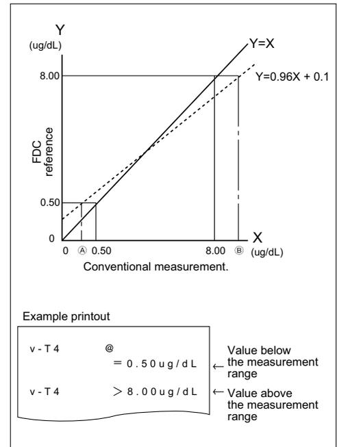
If the measured data is below the measurement range, a "@" indication is printed out, as shown at the top of the example printout.
