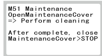
Open the maintenance door and clean the optical unit.
